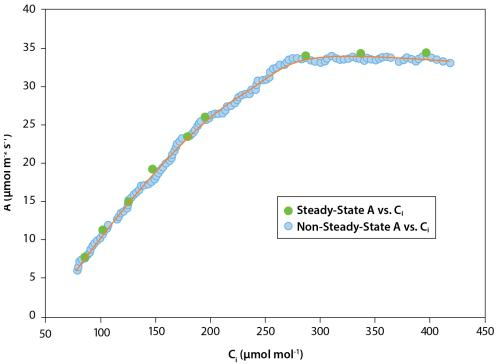
Comparison of a non-steady-state A/C<sub>i</sub> curve performed in 7 minutes using our high-speed CO<sub>2</sub> ramping technique to a traditional point-by-point steady-state A/C<sub>i</sub> curve performed in 35 minutes for a typical C<sub>3</sub> Bean (Phaseolus vulgaris) at 25 °C with PAR of 1800  $\mu$ mol m<sup>-2</sup> s<sup>-1</sup>.
