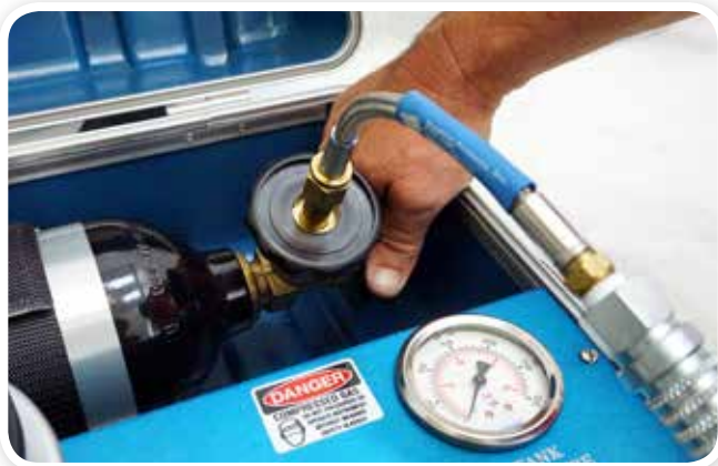
STEP 13: Open Model 615 tank just barely. You will hear a squealing sound. As the sounds lessens, open the valve slightly more. Continue this process till valve is completely open and pressure has equalized.
