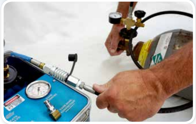
STEP 12: Hold end of 6-Foot Hose firmly in one hand. Open Valve slowly to pressurize hose.
