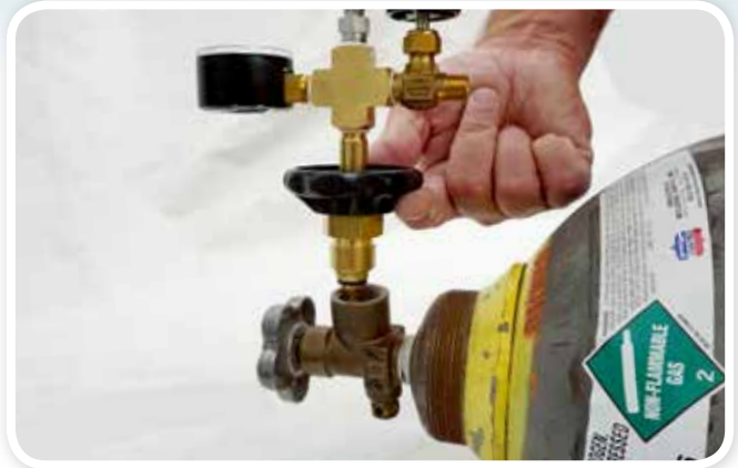
STEP 6: Screw the nitrogen connection of the 6-Foot Filling Hose into the Supply Tank Valve.
