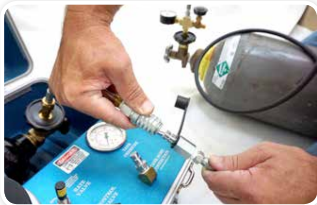
STEP 7: Align the end of the 6-Foot Filling Hose with the Model 615 tank hose and press the two fittings together.
