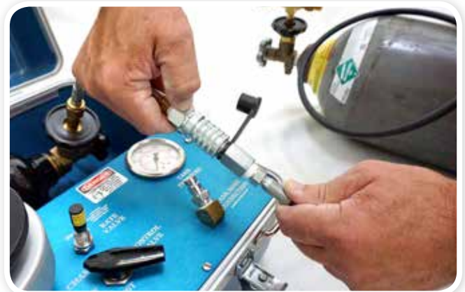
STEP 8: Ensure that quick connectors snap together. Pull gently on both hoses to ensure connection is secure.
