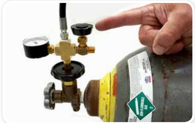
STEP 14: Close Model 615 Tank valve. Close Supply Tank Valve. Open Exhaust Valve to release pressure from 6 Foot Filling Hose.
