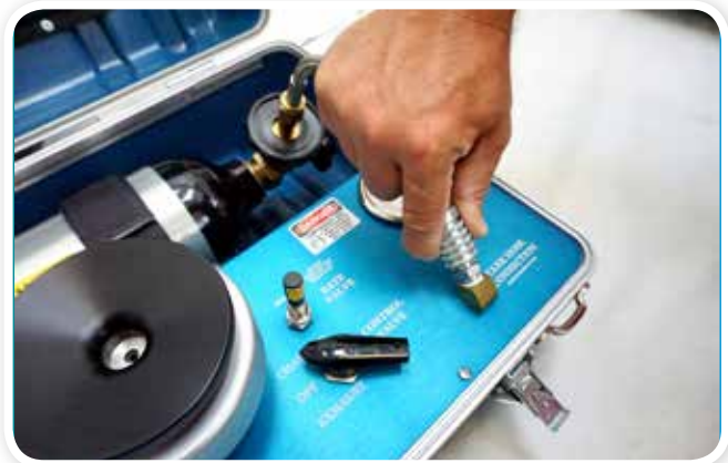
STEP 16: Connect Model 615 Tank Hose to the instrument side. Ensure properly connected by slight tug on hose.
