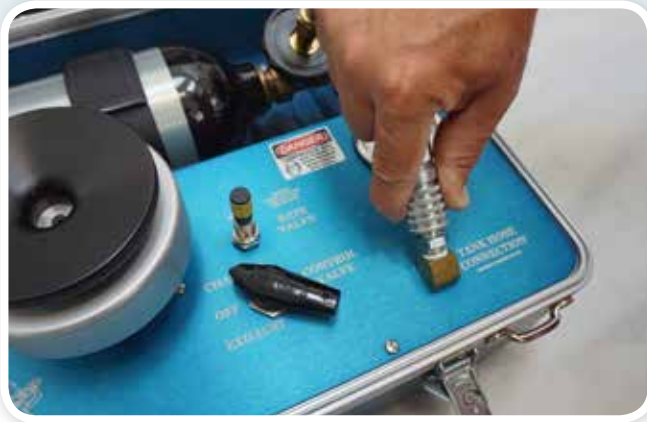
STEP 5: Firmly pull back on the outer sleeve of the Safety Quick Coupler to release from the instrument.
