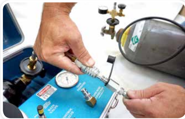
STEP 15: Disconnect 6-Foot Filling hose by pulling back on Safety Coupler on Model 615 Tank Hose.
